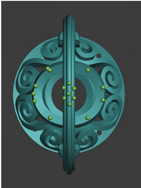
Figure 8. Anchor points added to starting point 2nd and 3rd bands of the ring.
