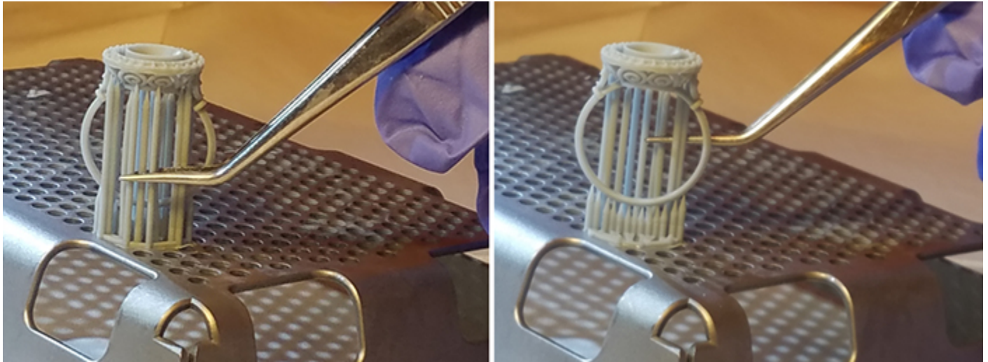
Figure 9. Removing side supports on the print platform.
