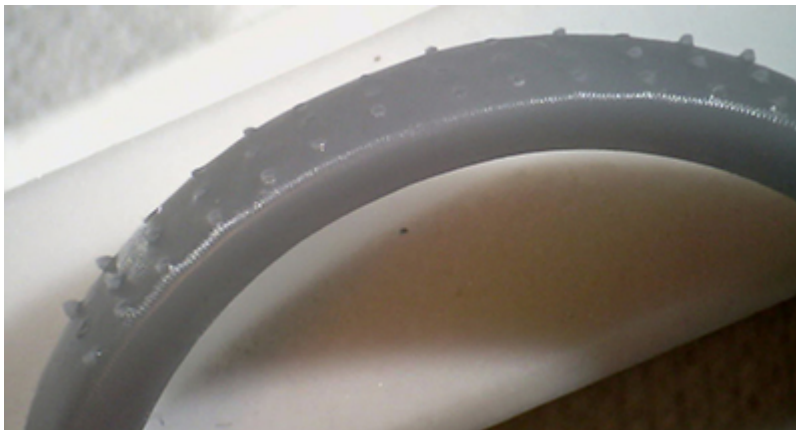
Figure 12. Magnified image of positive support nibs on the bottom of a ring.
