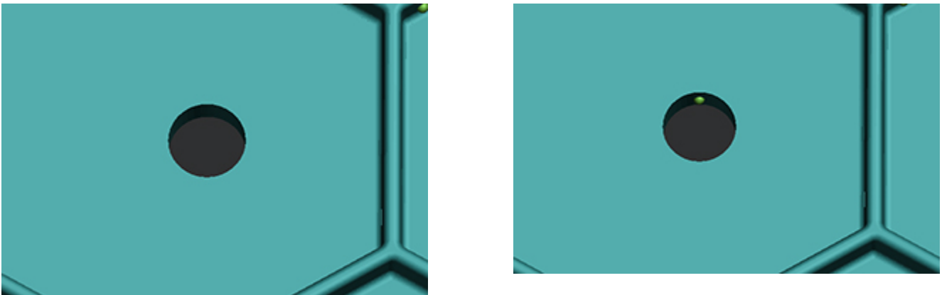
Figure 27. Default Fine Flat Tip anchor points are on the left where the hole has no supports. The image on the right side has one support added to the top inside edge of the hole.
